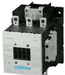
CONTACTOR, 55KW/400V/AC-3, AC(40...60HZ)/DC OPERATION UC 220...240V AUX. CONTACTS 2NO+2NC, 3-POLE, SIZE S6 BAR CONNECTIONS CONVENTIONAL OPERATING MECHAN. SCREW TERMINAL
