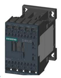
CONTACTOR, AC-3, 3KW/400V, 1NO, DC 24V, 0.85...1.85\*US, W. INTEGRATED VARISTOR 3-POLE SZ S00, SPRING-LOADED TERMINAL
