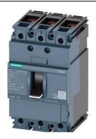
CIRCUIT BREAKER 3VA1 IEC FRAME 160 BREAKING CAPACITY CLASS N ICU=25KA @ 415 V 3-POLE, LINE PROTECTION TM210, FTFM, IN=160A OVERLOAD PROTECTION IR=160A FIXED SHORT CIRCUIT PROTECTION II=10 X IN BUSBAR CONNECTION
