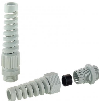
Metric cable glands with anti-kink protection MBFK, polyamide, light grey, IP 68 (5 bar, 30 min)
