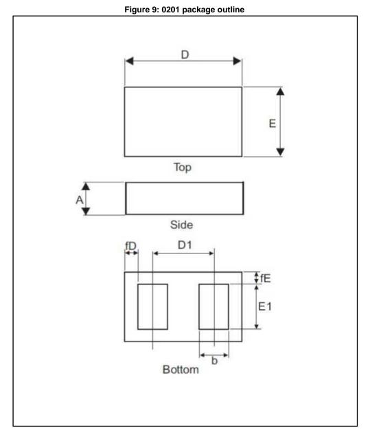
The marking codes can be rotated by 90 ° or 180° to differentiate assembly location. In no case should this product marking be used to orient the component for its placement on a PCB. Only pin 1 mark is to be used for this purpose.
