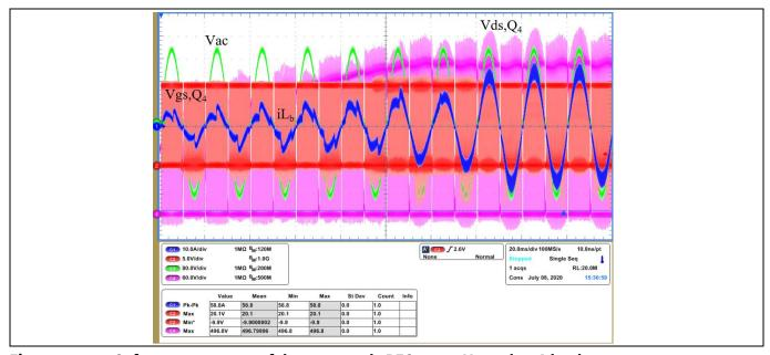
Figure 23 Soft-start sequence of the totem pole PFC at 180 V<sub>AC</sub> and 55 A load
