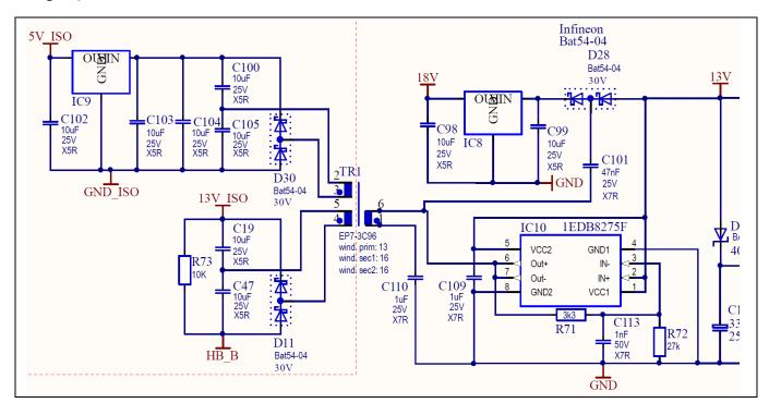
Proposed auxiliary supply circuit implemented with the single-channel driver 1EDB8275F Figure 51
