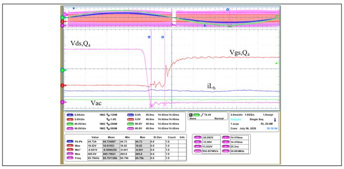
Figure 16 ZVS switch-on of the boost diode
