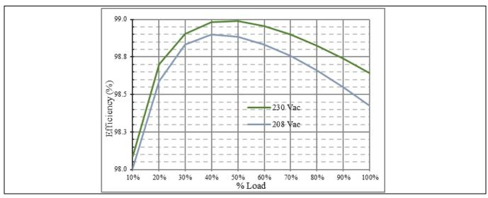
Figure 7 Estimated efficiency of the totem pole front-end AC-DC converter
