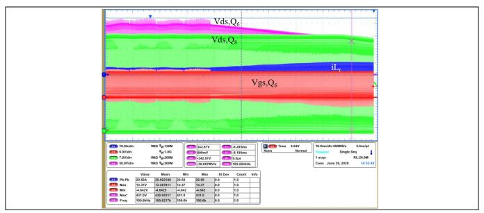
Figure 36 Brown-out sequence of the LLC converter at 10 A load while integrated into the complete **PSU**
