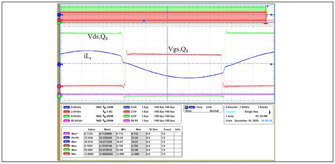
Figure 26 SRs gate driving at 40 A load and 410 V input voltage
