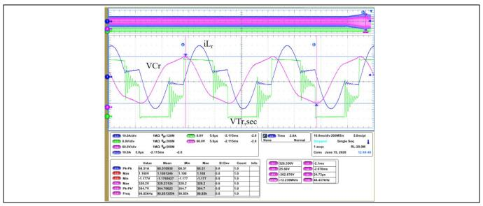
Figure 34 Clamping diodes limit the maximum V<sub>cr</sub> voltage amplitude, and therefore the gain of the converter
