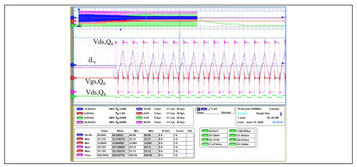
Figure 30 Detail view of the first pulses of the soft-start sequence
