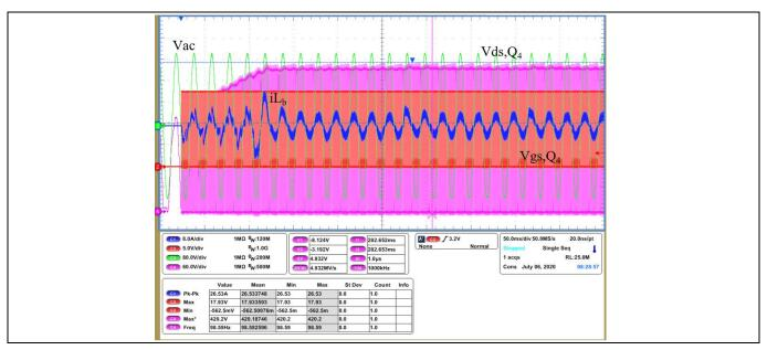
Figure 22 Soft-start sequence of the totem pole PFC at 180 V<sub>AC</sub> and 10 A load
