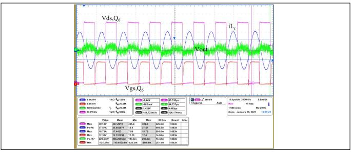
Figure 32 Output voltage ripple at full load
