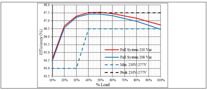
Figure 2 OCP rectifier V3 efficiency requirements at 230 V<sub>AC</sub> and estimated efficiency curve of a compliant PSU
