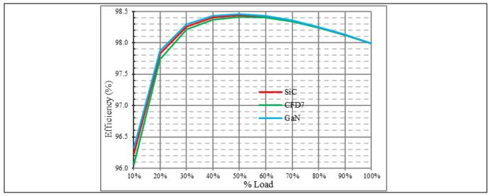
Figure 10 Estimated efficiency of the back-end LLC DC-DC converter
