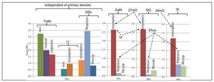
Figure 11 Estimated overall distribution of loss of the back-end LLC DC-DC converter at 50 percent load
