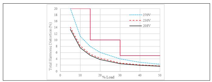
Figure 43 Measured THD of the complete power supply at several input voltages. The specification limits are shown in red.
