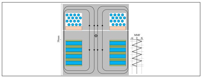
Figure 13 Simplified construction of the integrated transformer plus the parallel resonant inductor of the LLC DC-DC converter
