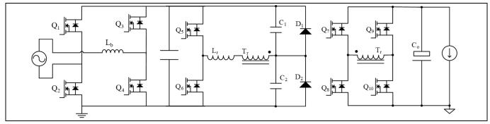
Figure 6 Simplified schematic of the EVAL\_3KW\_50V\_PSU. Front-end totem pole PFC followed by a half-bridge LLC resonant converter.
