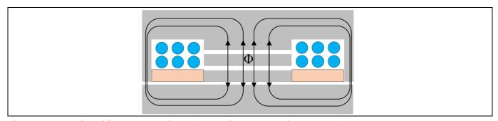
Figure 12 Simplified construction of the series resonant inductor of the LLC DC-DC converter
