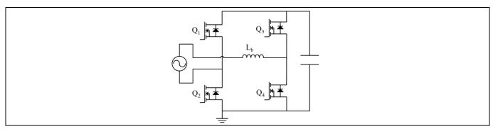
Figure 4 Simplified schematic of the totem pole AC-DC converter (EVAL\_3K3W\_TP\_PFC\_SIC)
