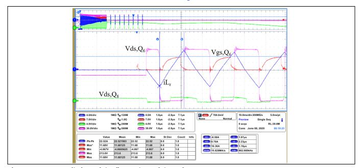
Figure 31 Detail view of the first pulses of the soft-start sequence
