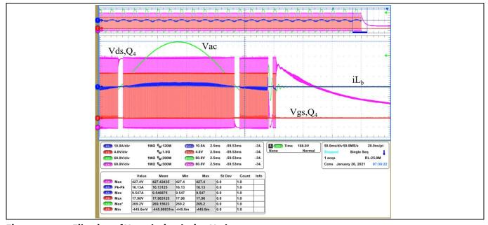
Figure 21 Filtering of V<sub>AC</sub> polarity during V<sub>AC</sub> loss
