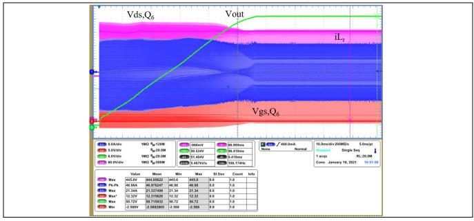
Figure 29 Soft-start sequence at 40 A load
