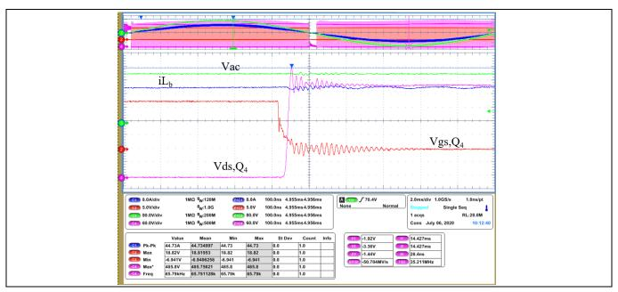
Figure 18 Hard-switched turn-off of the boost switch
