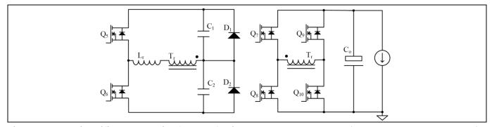
Figure 5 Simplified schematic of the half-bridge LLC DC-DC converter (EVAL\_3K3W\_LLC\_HB\_CFD7)
