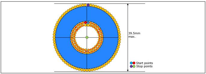
Figure 9 Simplfied recommended building instructions for the main boost inductor
