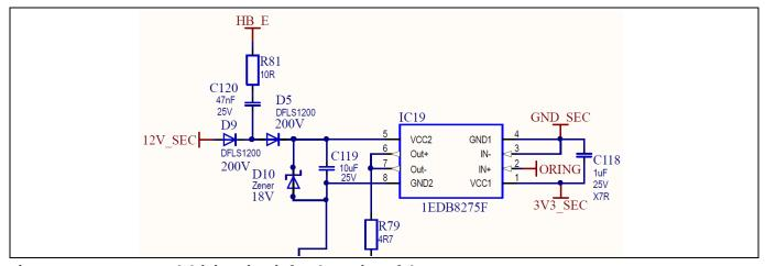
Figure 49 Proposed driving circuit for the ORing of the PSU
