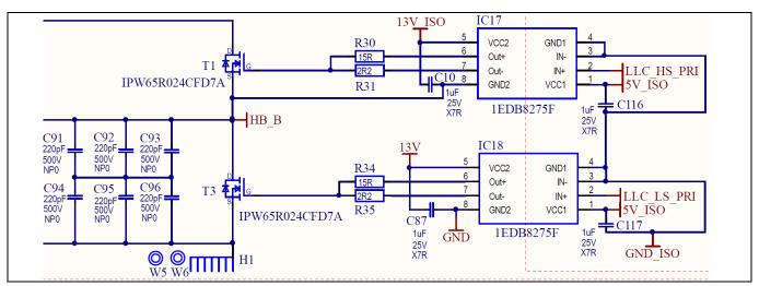
Figure 48 Recommended driving circuitry for the primary-side devices in the half-bridge LLC
