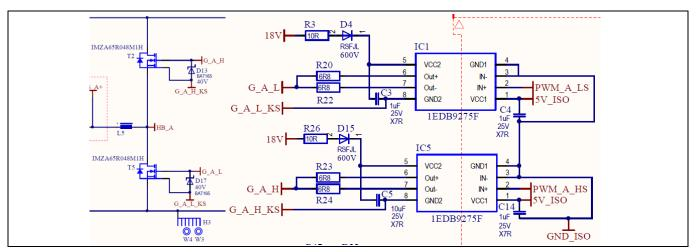
Figure 46 Recommended driving circuitry for the boosting half-bridge in the totem pole PFC
