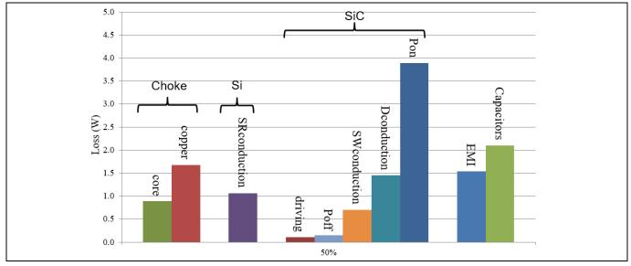
Estimated overall distribution of loss in the totem pole PFC at 230 V<sub>AC</sub> and 50 percent of the Figure 8 load
