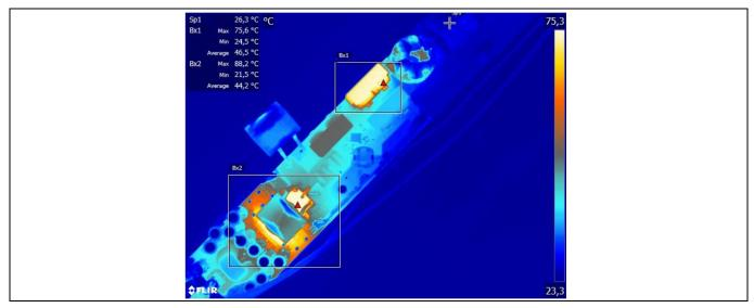
Figure 39 Measured temperature of the complete power supply prototype at full load, 230 V<sub>AC</sub> and outside of its chassis
