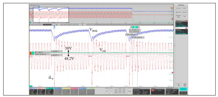
Figure 37 Detail view of 20 ms hold-up time at 60 A load and 230  $V_{AC}$
