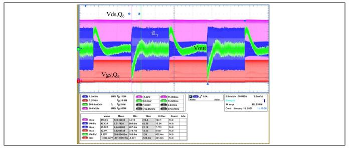
Figure 33 Dynamic load jump 10 A load to 40 A load, 1 A/μs, 100 Hz
