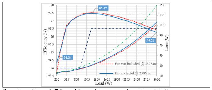
Figure 41 Measured efficiency of the complete power supply prototype at 230 V<sub>AC</sub>
