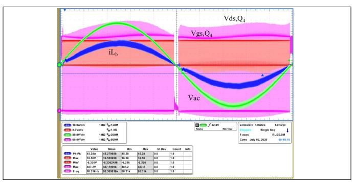
Figure 15 PFC drain voltage overshoot and gate ringing at full load
