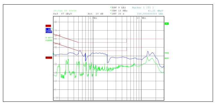
Figure 45 Measured EMI spectrum of the complete power supply prototype at 230 V<sub>AC</sub> and 2.5 kW. Quasi-peak is shown in blue and average in green.
