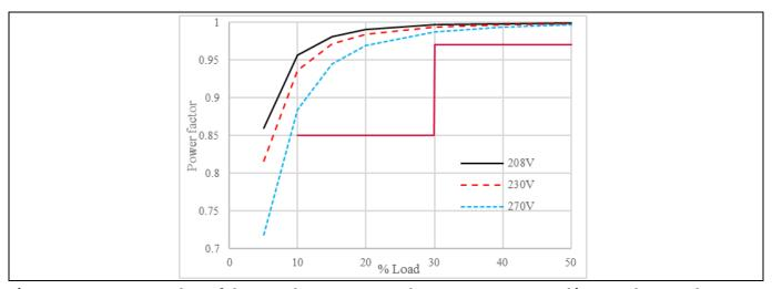
Measured PF of the complete power supply prototype at several input voltages. The Figure 42 specification limits are shown in red.
