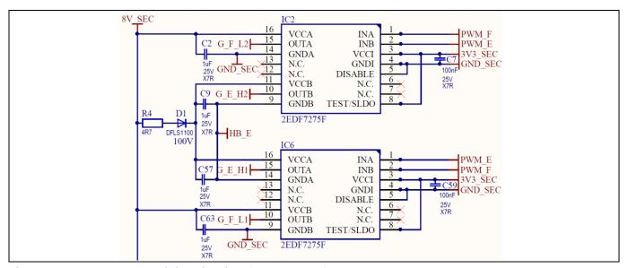
Figure 50 Proposed driving circuitry for the SRs of the LLC DC-DC converter
