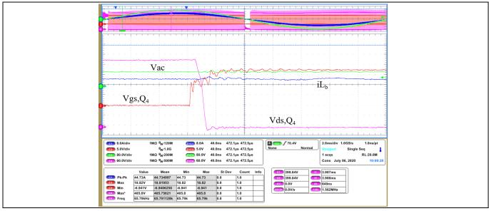
Hard-swiched turn-on of the boost switch and hard-commutation of the boost diode Figure 19
