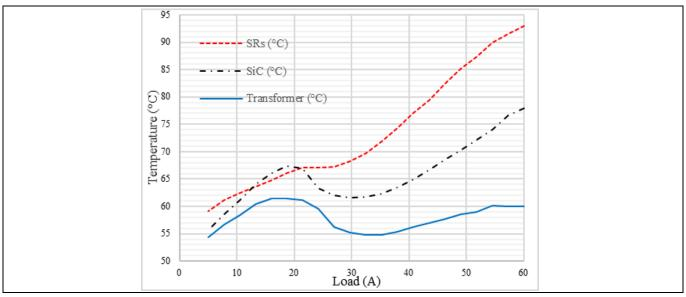
Figure 40 Measured temperature of the complete power supply prototype at full load, 180 V<sub>AC</sub> and inside of its chassis
