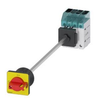
Switch disconnector 3LD3, main switch 3-polig + N, lu 40A operational switch at AC-23 A at 400 V 15,0 kW floor mounting Base mounting with door coupling center-hole 22,5 mm knob-operated mechanism red/yellow 48 x 48 mm
