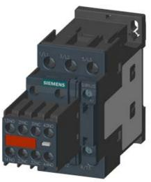
CONTACTOR, AC-3, 11KW/400V, 2NO+2NC, AC 230V 50/60HZ, W. PLUGGED-IN VARISTOR 3-POLE, SZ S0 SCREW TERMINAL PERMANENT AUX. SWITCH
