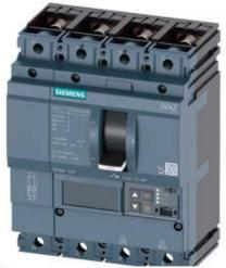
CIRCUIT BREAKER 3VA2 IEC FRAME 100 BREAKING CAPACITY CLASS L ICU=150KA @ 415 V 4POLE, LINE PROTECTION ETU850, LSI, IN=40A OVERLOAD PROTECTION IR=16A ...40A SHORT CIRCUIT PROTECTION ISD=0,6..10X IN, II=1,5..12X IN NEUTRAL PROTECTION ADJUSTABLE (OFF, UPTO 160%) BUSBAR CONNECTION
