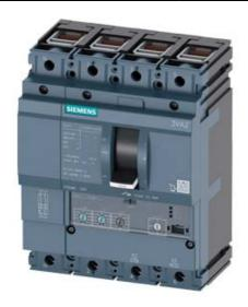
CIRCUIT BREAKER 3VA2 IEC FRAME 160 BREAKING CAPACITY CLASS C ICU=110KA @ 415 V 4POLE, LINE PROTECTION ETU320, LI, IN=25A OVERLOAD PROTECTION IR=10A ...25A SHORT CIRCUIT PROTECTION II=12 X IN NEUTRAL PROTECTION ADJUSTABLE(OFF,100%) CABLE CONNECTION
