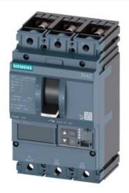
CIRCUIT BREAKER 3VA2 IEC FRAME 250 BREAKING CAPACITY CLASS L ICU=150KA @ 415 V 3POLE, LINE PROTECTION ETU550, LSI, IN=250A OVERLOAD PROTECTION IR=100A ...250A SHORT CIRCUIT PROTECTION ISD=0,6..10X IN, II=1,5..10X IN NEUTRAL PROTECTION OPTIONAL WITH EXT. CT,UPTO 160% BUSBAR CONNECTION
