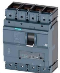
CIRCUIT BREAKER 3VA2 IEC FRAME 630 BREAKING CAPACITY CLASS M ICU=55KA @ 415 V 4-POLE, LINE PROTECTION ETU350, LSI, IN=400A OVERLOAD PROTECTION IR=160A ...400A SHORT CIRCUIT PROTECTION ISD=1,5... 10 X IR, II=12 X IN NEUTRAL PROTECTION ADJUSTABLE(OFF,50%,100%) BUSBAR CONNECTION
