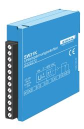
Undervoltage monitor for threephase networks without N for monitoring on voltage failure. The voltage is being measured between phases and an artificial neutral point. At symmetrical decrease of the voltage to approx. 50% of the nominal value or in case of failure of a phase the integrated relay (1 change-over contact) releases with a delay of approx. 1s. With engines runningon on 2 phases, so much back voltage can be produced that the failure of a phase may be
