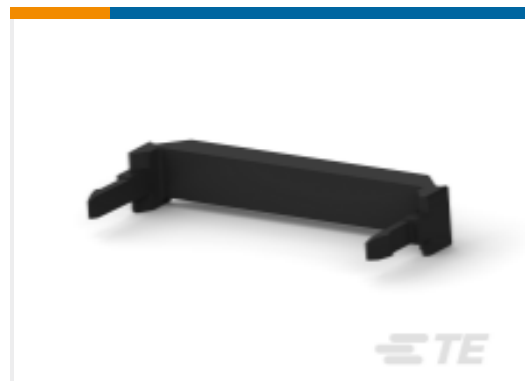
TE Part #1-499252-2 Bus Connector: Strain Relief, ATA
