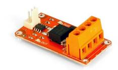
**Module Description**: This module features an IRF520 power MOSFET transistor, a kick-back diode, a standard TinkerKit 3pin connector, a signal amplifier, a green LED that signals that the module is correctly powered and one yellow LED whose brightness depends on the input signal received by the module.
