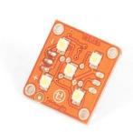
This module is an **ACTUATOR**. The connector is an **INPUT** which must be connected to an **OUTPUT** connector on the **TinkerKit Shield**.
