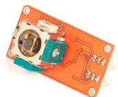
**Module Description**: This module features two 4k7 Ohm linear potentiometers, two standard TinkerKit 3pin connector, two signal amplifiers, a green LED that signals that the module is correctly powered and two yellow LED whose brightness depends on the values output by the module.
