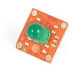
The **LED** is possibly the simplest actuator available. It's a low power light source available in many colors. It lights up when powered from an Arduino pin.
