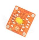
The **LED** is possibly the simplest actuator available. It's a low power light source available in many colors. It lights up when powered from an Arduino pin.
