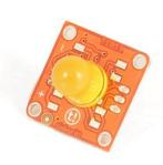
that the module is correctly powered and a tiny yellow LED that shows the current brightness of the yellow LED. A resistor provides the optimal amount of current when connected to an Arduino.
