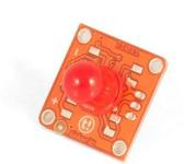
This module is an **ACTUATOR** therefore the connector is an INPUT that need to be connected to one of the **OUTPUT** connectors on the **TinkerKit Shield**.
