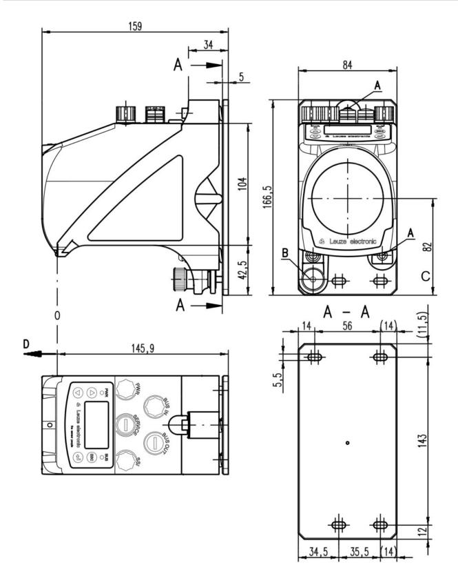
A M 5 screw for alignment B Knurled nut with WAF 4 hexagon socket and M 5 nut for securing
