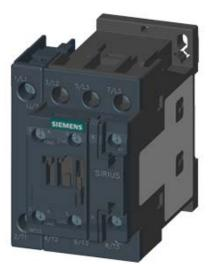
4NO CONTACTOR, AC1: 35A AC 230V 50/60HZ 4-POLE, 4NO, SZ: S0, SCREW TERMINAL 1NO+1NC INTEGR.
