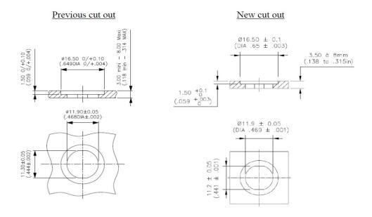
IXP will be compliant with the previous panel cut out, IXR can be mounted on the new panel cut out.
