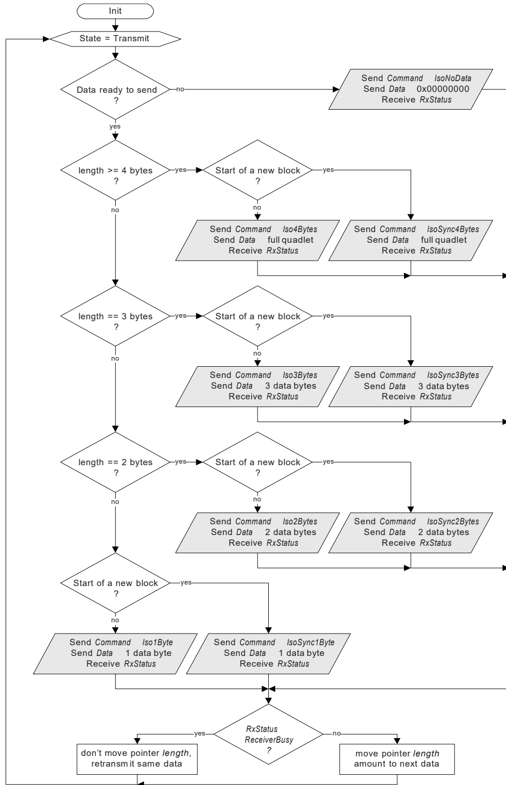
Figure 48-14. Isochronous Data Tx Device Protocol
