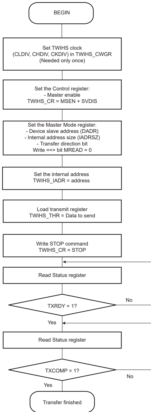
Figure 43-15. TWIHS Write Operation with Single Data Byte and Internal Address
