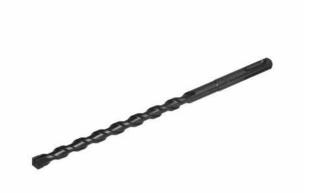
$\sim$  Tungsten carbide tipped with optimized geometry for drilling concrete and stone  $\sim$  Vacuum brazed tips for durability  $\sim$  Ground flutes designed for optimum debris removal  $\sim$  SDS-plus shank  $\sim$  Diameter: 4 mm  $\sim$  Working length: 48 mm  $\sim$  Total length: 110 mm Features & Benefits
