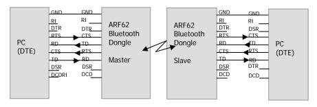
SPP configuration guideline: in the following example, the Master is configured to performed an auto-connection on reset.
