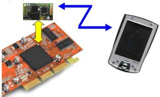
The A<sup>RF62</sup> dongle fully complies with the V2 Bluetooth® standard and air data rate goes up to 723 kbps. Data exchange and set-up are only done through an UART data port, under SPP or DUN profile. A miniature antenna is integrated.
