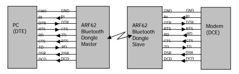
DUN configuration guideline : in the following example, the Master is configured to performed an auto-connection on DSR.
