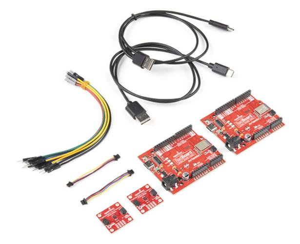
With the SparkFun Cryptographic Development Kit you will get everything you need to learn the fundamentals of cryptographic authentication and how to use the ATECC508A Cryptographic Co-Processor Breakout to add a soaring level of security to your projects.
