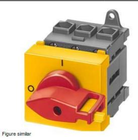
MAIN/EMERG. STOP SWITCH 3-POLE IU=32, P/AC-23A AT 400V=11.5KW FLOOR MOUNTING DIN RAIL/TWO-HOLE MOUNTING KNOB RED/YELLOW (EMERG. STOP)
