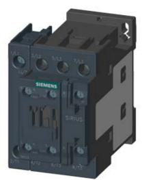
4NO CONTACTOR, AC1: 35A AC 230V 50/60HZ 4-POLE, 4NO, SZ: S0, SCREW TERMINAL 1NO+1NC INTEGR.
