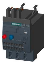
OVERLOAD RELAY 7.0...10 A FOR MOTOR PROTECTION SZ S00, CLASS 10, F. MOUNTING ONTO CONTACTOR MAIN CIRCUIT: SPRING TERMINAL AUX. CIRCUIT: SPRING TERMINAL MANUAL-AUTOMATIC-RESET
