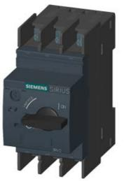
CIRCUIT-BREAKER SZ S00, FOR MOTOR PROTECTION, CLASS 10, A-RELEASE 2.8...4A, N-RELEASE 52A, RING CABLE LUG CONNECTION, STANDARD SW. CAPACITY
