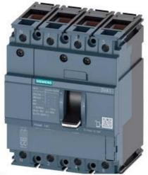
CIRCUIT BREAKER 3VA1 IEC FRAME 160 BREAKING CAPACITY CLASS M ICU=55KA @ 415 V 4-POLE, LINE PROTECTION TM210, FTFM, IN=20A OVERLOAD PROTECTION IR=20A FIXED SHORT CIRCUIT PROTECTION II=10 X IN NEUTRAL PROTECTION 100% CABLE CONNECTION
