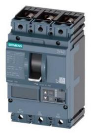
CIRCUIT BREAKER 3VA2 IEC FRAME 160 BREAKING CAPACITY CLASS H ICU=85KA @ 415 V 3POLE, LINE PROTECTION ETU550, LSI, IN=160A OVERLOAD PROTECTION IR=64A ...160A SHORT CIRCUIT PROTECTION ISD=0,6..10X IN, II=1,5..10X IN NEUTRAL PROTECTION OPTIONAL WITH EXT. CT,UPTO 160% BUSBAR CONNECTION
