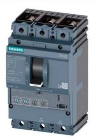
CIRCUIT BREAKER 3VA2 IEC FRAME 160 BREAKING CAPACITY CLASS H ICU=85KA @ 415 V 3POLE, LINE PROTECTION ETU350, LSI, IN=63A OVERLOAD PROTECTION IR=25A ...63A SHORT CIRCUIT PROTECTION ISD=1,5... 10 X IR, II=12 X IN BUSBAR CONNECTION
