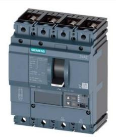
CIRCUIT BREAKER 3VA2 IEC FRAME 160 BREAKING CAPACITY CLASS H ICU=85KA @ 415 V 4POLE, LINE PROTECTION ETU850, LSI, IN=63A OVERLOAD PROTECTION IR=25A ...63A SHORT CIRCUIT PROTECTION ISD=0,6..10X IN, II=1,5..12X IN NEUTRAL PROTECTION ADJUSTABLE (OFF, UPTO 160%) BUSBAR CONNECTION
