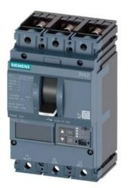
CIRCUIT BREAKER 3VA2 IEC FRAME 250 BREAKING CAPACITY CLASS L ICU=150KA @ 415 V 3POLE, LINE PROTECTION ETU860, LSIG, IN=160A OVERLOAD PROTECTION IR=64A ...160A SHORT CIRCUIT PROTECTION ISD=0,6..10X IN, II=1,5..12X IN NEUTRAL PROTECTION OPTIONAL WITH EXT. CT,UPTO 160% GROUNDFAULT, SWITCHABLE IG=0,2... 1 X IN, TG=0,050,8MS BUSBAR CONNECTION
