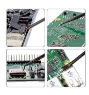
Experience precise and improved soldering with Weller's Solder Aid Kit with 6 Double-sided Tools that offer multi-functional capabilities. Use to bend and hold leads, remove dust and contamination, adjust pins and components, and many other necessary tasks.
