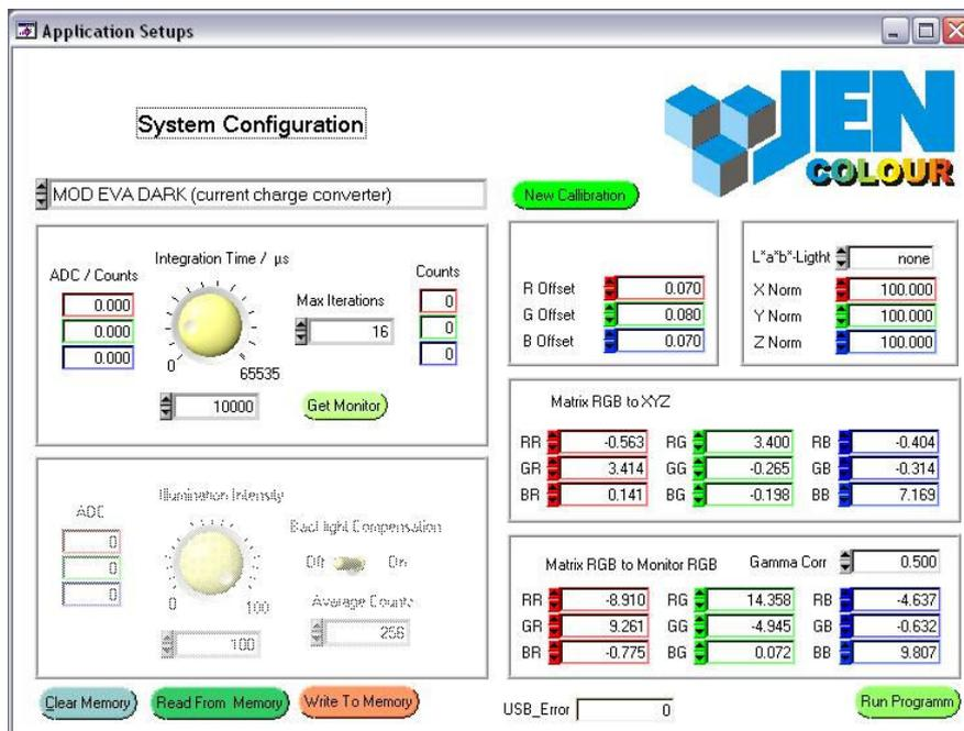
Figure 22: Sample configuration for modEVA-DARK (current-to-charge converter)
