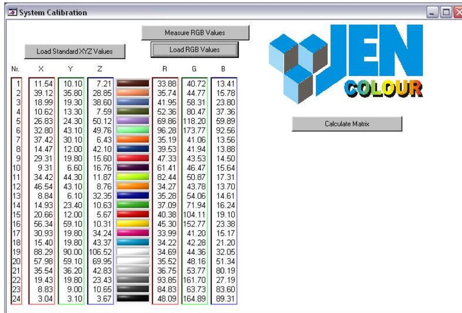
Figure 29: System calibration – calculation of matrix
