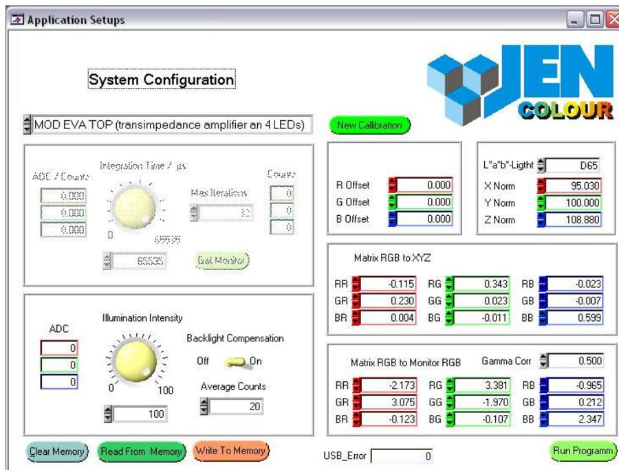
Figure 23: Sample configuration with modEVA-TOP
