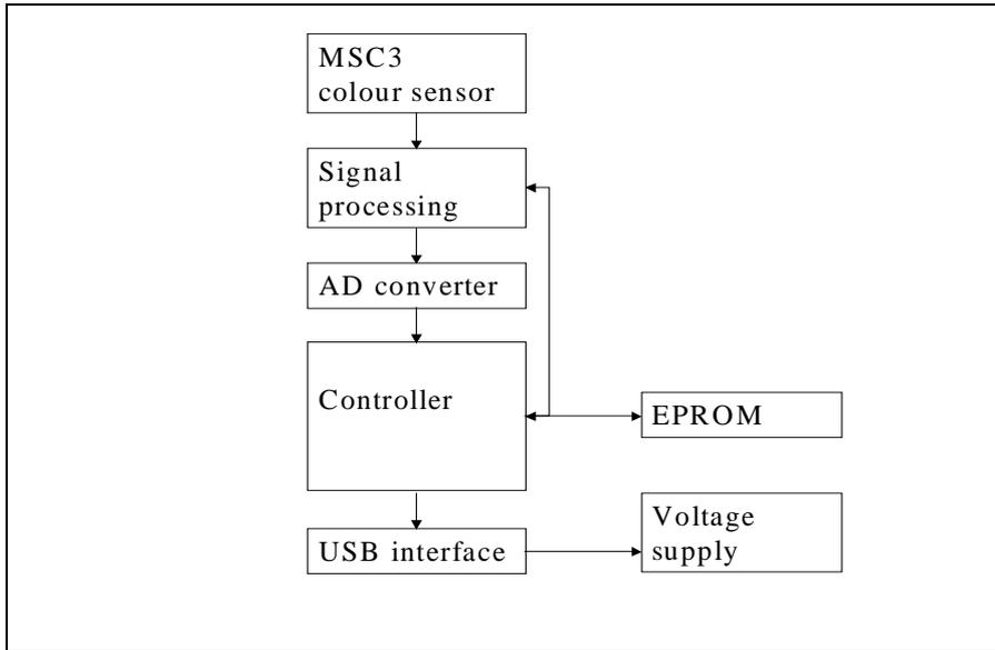
Figure 4: Block diagram of MTCS-MEK
