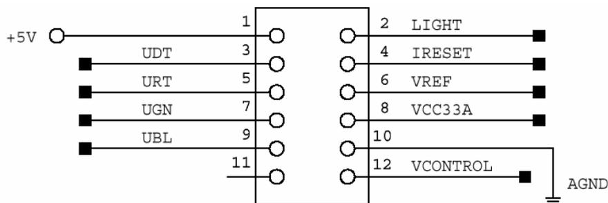
Figure 6: Signal assignments of sensor interface
