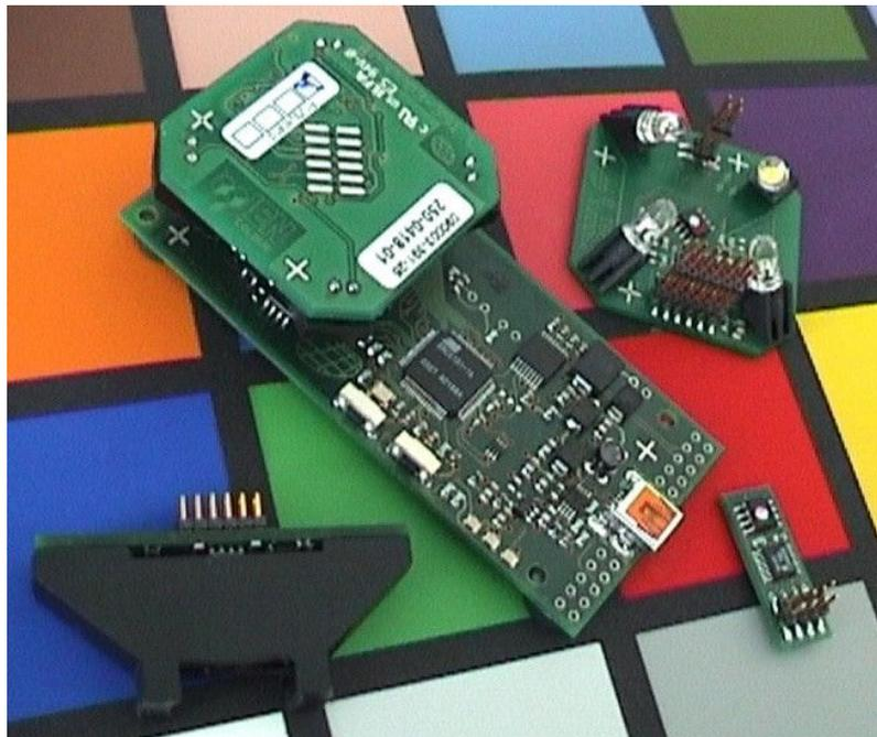
Figure 1: MTCS-ME1 mainboard with sensor module mounted
