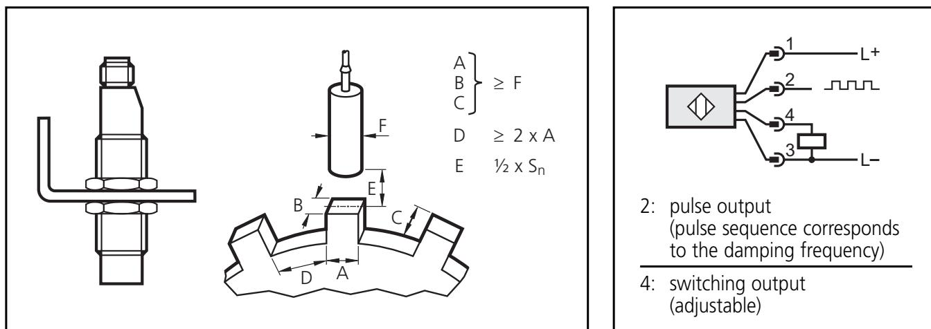
Fix the unit by means of a mounting fixture and protect it against loosening by means of the enclosed nuts. Not flush mountable.
