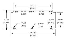
Enclosures can be Factory Modified (Milling, Drilling, Printing etc. Contact Factory mjm@hammondmfg.com for quotes Solid models of this enclosure available in STEP or IGES.
