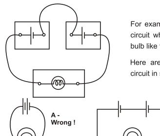
For example, in experiment 2 you set up a circuit which had 2 cells connected to one bulb like this:-
