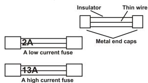
Equipment such as electrical heaters take a large current so are fitted with thick wire fuses, e.g. "13 amp", but low current equipment such as lights or a television set need a thinner wire fuse, e.g. "2 amp".
