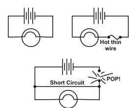
In this simple circuit the electricity has to flow through the bulb. If you look at a bulb closely you will see that the electricity passes through an extremely thin wire called a FILAMENT. As you have already learned, very thin wires have a very high resistance than thick wires. So this resistance will keep the electrical current down to a safe value.
