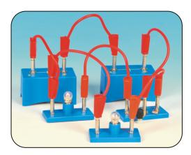
Set up the circuit shown here with two changeover switches. This circuit is unusual in that two switches are used to control only one light bulb.
