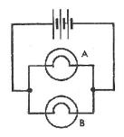
Use two switches in this circuit so that when one switch is pressed, lamp A lights up and when the other switch is pressed, lamp B lights up.
