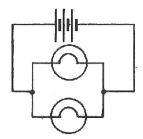
Place a switch so that one lamp stays on all the time but the other only lights when the switch is pressed.
