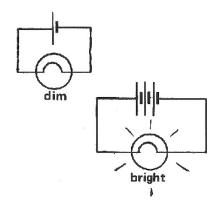
In several experiments so far you have found that you can increase the "driving force" of a battery by adding more cells in series, the more current flows round a circuit. In the last experiment, we learned how to use an AMMETER to measure the CURRENT round a circuit.
