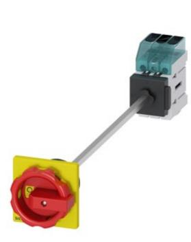
Switch disconnector 3LD3, main switch 3-polig, lu 63A operational switch at AC-23 A at 400 V 22,0 kW floor mounting Base mounting with door coupling center-hole 22,5 mm rotary operationg mechanism red/yellow 66 x66 mm
