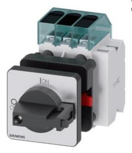
Switch disconnector 3LD3, main switch 3-polig, lu 63A operational switch at AC-23 A at 400 V 22,0 kW front mounted Base mounting with center-hole 22,5 mm knob-operated mechanism black 48 x 48 mm with auxiliary 1NO+1NC
