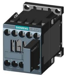
COUPLING CONTACTOR RELAY, 2NO+2NC, DC 24V, 0.7...1.25\*US, W/ PLUGGED-ON VARISTOR, SIZE S00, SCREW TERMINAL
