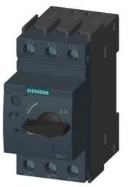
SPECIAL TYPE CIRCUIT BREAKER SIZE S00, FOR TRANSFORMER PROTECTION A-RELEASE 7...10A, SHORT-CIRCUIT RELEASE 208A, SCREW TERMINAL, STANDARD SWITCHING CAPACITY AMBIENT TEMPERATURE -50 DEGREES C 500 SWITCHING CYCLES
