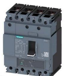
CIRCUIT BREAKER 3VA1 IEC FRAME 160 BREAKING CAPACITY CLASS M ICU=55KA @ 415 V 4-POLE, LINE PROTECTION TM220, ATFM, IN=160A OVERLOAD PROTECTION IR=112A ...160A SHORT CIRCUIT PROTECTION II=10 X IN NEUTRAL PROTECTION 50% BUSBAR CONNECTION
