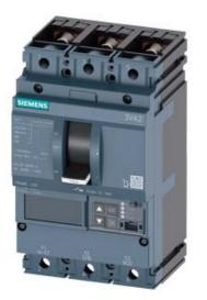
CIRCUIT BREAKER 3VA2 IEC FRAME 100 BREAKING CAPACITY CLASS C ICU=110KA @ 415 V 3POLE, LINE PROTECTION ETU560, LSIG, IN=25A OVERLOAD PROTECTION IR=10A ...25A SHORT CIRCUIT PROTECTION ISD=0,6..10X IN, II=1,5..12X IN NEUTRAL PROTECTION OPTIONAL WITH EXT. CT,UPTO 160% GROUNDFAULT, SWITCHABLE IG=0,2... 1 X IN, TG=0,050,8MS BUSBAR CONNECTION
