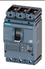
CIRCUIT BREAKER 3VA2 IEC FRAME 250 BREAKING CAPACITY CLASS H ICU=85KA @ 415 V 3POLE, LINE PROTECTION ETU860, LSIG, IN=160A OVERLOAD PROTECTION IR=64A ...160A SHORT CIRCUIT PROTECTION ISD=0,6..10X IN, II=1,5..12X IN NEUTRAL PROTECTION OPTIONAL WITH EXT. CT,UPTO 160% GROUNDFAULT, SWITCHABLE IG=0,2... 1 X IN, TG=0,050,8MS BUSBAR CONNECTION
