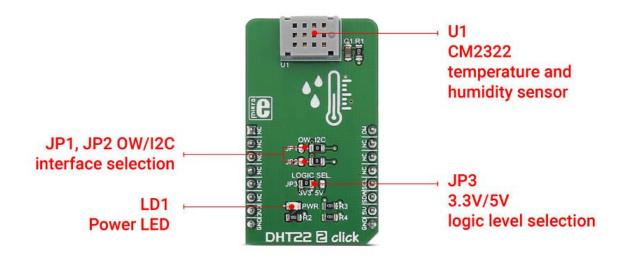
Typical temperature accuracy is  $\pm 0.3^{\circ}$ C, while relative humidity accuracy is 2% RH, with the resolution of 0.1 for both measured properties. I2C/1-Wire interface is used to communicate with the host MCU, sending the measurement data every 2 seconds. Proprietary data collecting techniques are used to average the sampled values, after which the result is sent via the I2C/1-Wire bus.
