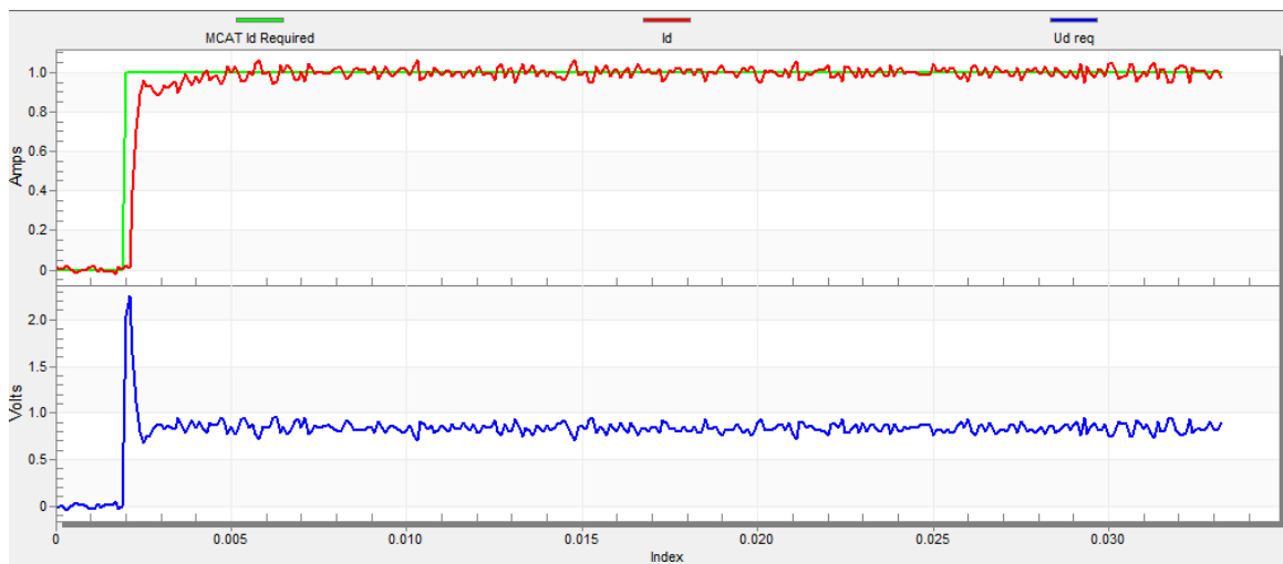
Figure 26. Optimal step response of Id current controller
