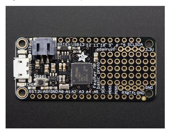
At the Feather M0's heart is an ATSAMD21G18 ARM Cortex M0 processor, clocked at 48 MHz and at 3.3V logic, the same one used in the new Arduino Zero. This chip has a whopping 256K of FLASH (8x more than the Atmega328 or 32u4) and 32K of RAM (16x as much)! This chip comes with built in USB so it has USB-to-Serial program & debug capability built in with no need for an FTDI-like chip.
