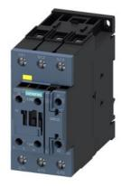
power contactor, AC-3e/AC-3, 80 A, 37 kW / 400 V, 3-pole, 175-280 V AC/DC, 50/60 Hz, with integrated varistor, auxiliary contacts: 1 NC, screw terminal, size: S2, F-PLC-IN
