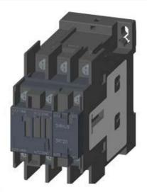
CONT. F. RAILWAY APPL., AC-3, 7.5KW/400V, 1NO+1NC, . DC 24V, 0.7...1.25\*US, W. VARISTOR INTEGRATED, 3-POLE SIZE S0, RING CABLE LUG CONNECTION
