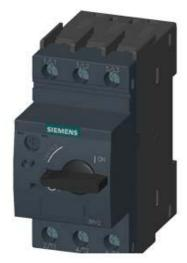
CIRCUIT-BREAKER SZ S0, FOR MOTOR PROTECTION, CLASS 10, A-REL. 0.45...0.63A, N-REL.8.2A SCREW CONNECTION, STANDARD SW. CAPACITY
