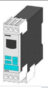
DIGITAL MONITORING RELAY VOLTAGE MONITORING, 22.5MM FROM 10 TO 600V AC/DC OVERSHOOT AND UNDERSHOOT AC/DC 24 TO 240V DC AND AC 50 TO 60 HZ SPIKE DELAY 0.1 TO 20S HYSTERESIS 0.1 TO 300V 1 CHANGEOVER CONTACT W. OR W/O ERROR LOG SCREW TERMINAL REPLACEMENT PRODUCT F. 3UG3532-1AL20, 3UG3532-1AG20
